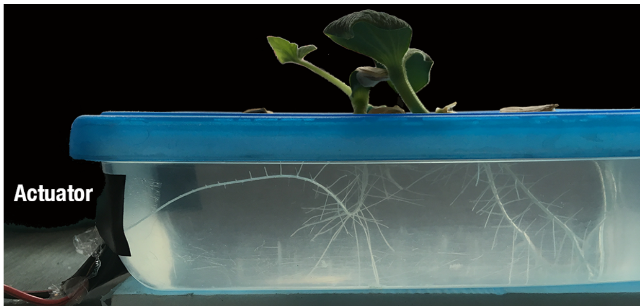
Figure 1: A prototype with an Arduino Uno driving a Tectonic Elements TEAX25C05-8 transducer with a 250 Hz sine wave. The image shows results of approximately two weeks of continuous stimulation on the root orientation of pumpkin seeds ( Cucurbita maxima ). One root can be observed to orient towards the source of vibration. Root growth would be expected to be more diffuse without stimulation, though, note, this is a single-trial result for illustration purposes.
